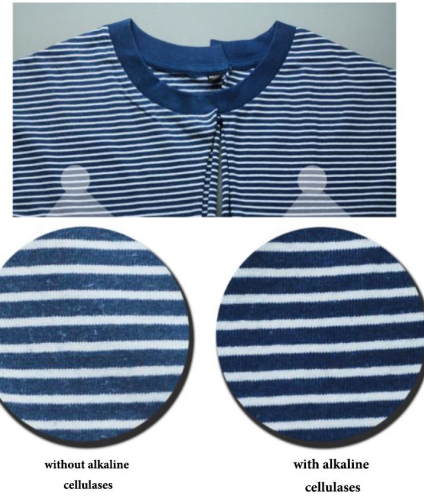
> Fig. 5 Effect of alkaline cellulase on the renovation of cotton striped shirts, the
